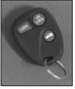
The remote keyless entry system consists of a receiver, which is located in the vehicle, and two hand held transmitters.
